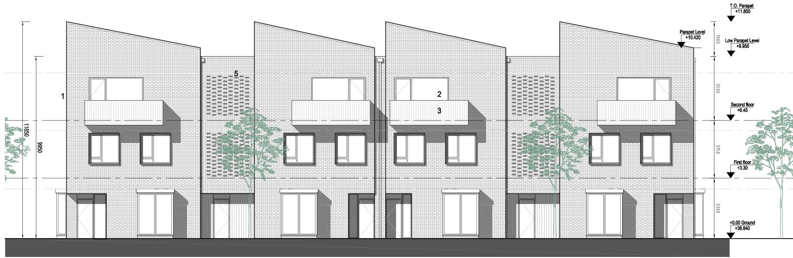
**FRONT ELEVATION** BLOCKS B1 AND B2 (BLOCK B1 FFL = 37.500, BLOCK B2 FFL = 37.000)
