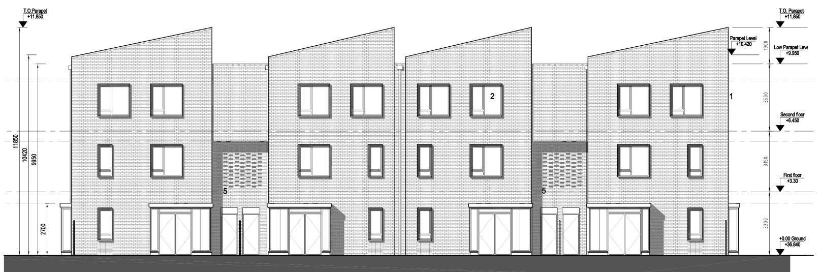
**REAR ELEVATION** BLOCKS B1 AND B2 (BLOCK B1 FFL = 37.500, BLOCK B2 FFL = 37.000)
